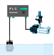
The bare wire overflow detector version, connected to a PLC, allows a change of status to be sent to the PLC, as well as a fouling indicator (if Modbus interface configured).
